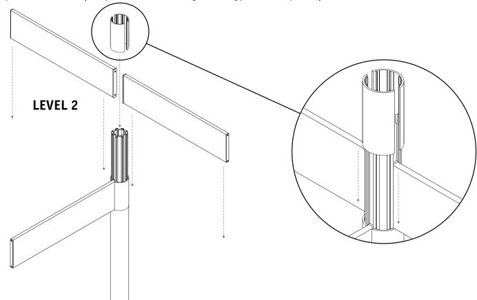
4. Slot the Beacon Cap onto the Extrusion and screw into place (Standard cap is optional with reduced inner extrusion)
