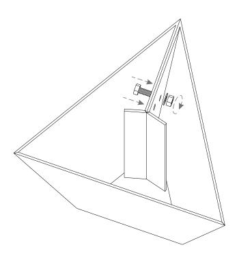
4. Mount the Marker Cone to the Post by passing the Screw Band through the rectangular holes. Then tighten the screwband with a spanner.
