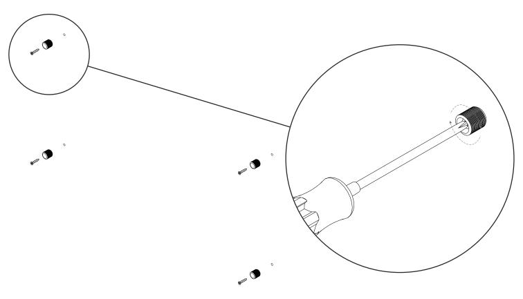
4. Screw Middle Section of the Stand off Locators onto the Back Section.
