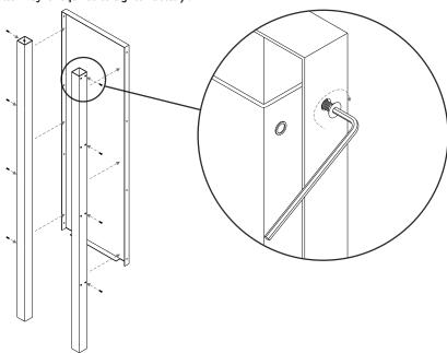
2. Slot the other tray into place and connect using the M6 Countersunk bolts into the Nut inserts in the internal posts.
