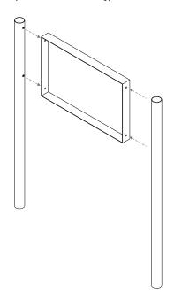
2. Use the bolts and washers to connect the Posts to the Tray ( Tighten with a spanner ) .
