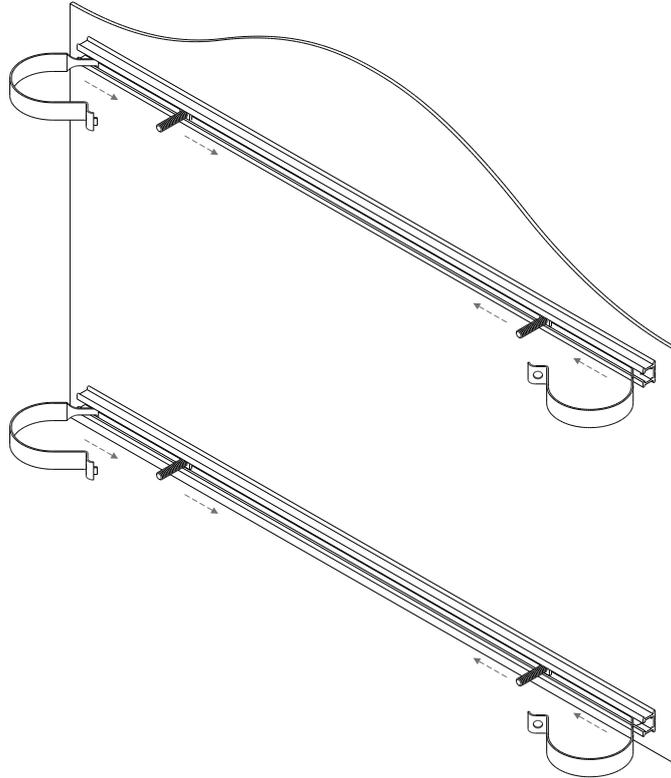
4. Place the Sign Panel (with channel) against the posts and place the clips around the posts then connect it to the bolt. Then use the spacer and nut to tighten the sign in position.
