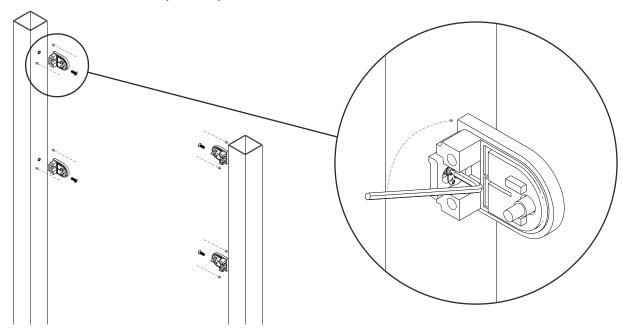
2. Place the Acrylic panel onto the mounted Glass Clamp (Back Section). Align holes with pins
