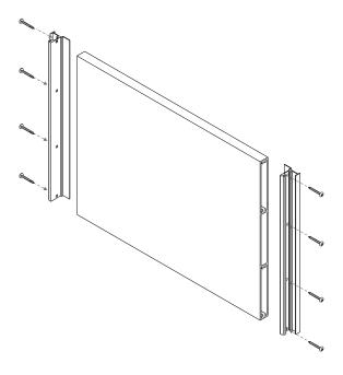
2. Position your Modular Sign on the wall (use a spirit level if required). Drill your holes in the side track and into the wall (use wall plugs if required).
