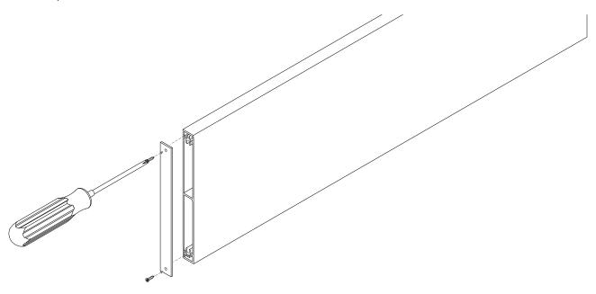
2. Screw the Wall Bracket onto the other end of the Modular Plank.
