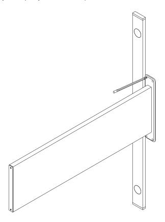
4. Drill the holes for mounting to the wall (add wall plugs if required).
