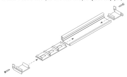
2. Holes will have to be drilled in the gaps of the Plastic Edge Clip and through the Edge Strip extrusion to mount to the wall.
