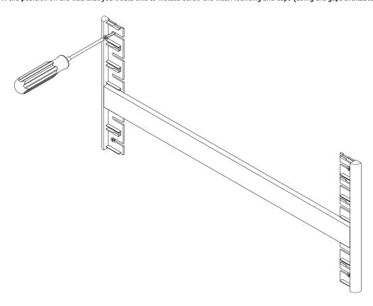
3. After the system as been screwed to the wall, you can simply push the other K'nect slats into position.
