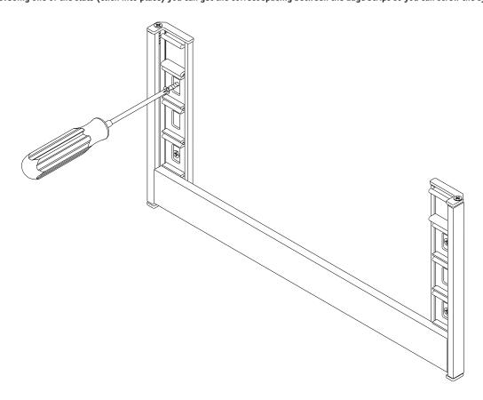
4. After the system as been screwed to the wall, you can simply push the other K'nect slats into position.
