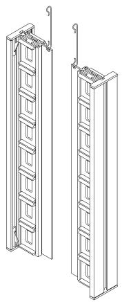
4. Connect the Slat Extrusions to both sides of the Suspended Edge Strip Extrusion (as shown below).
