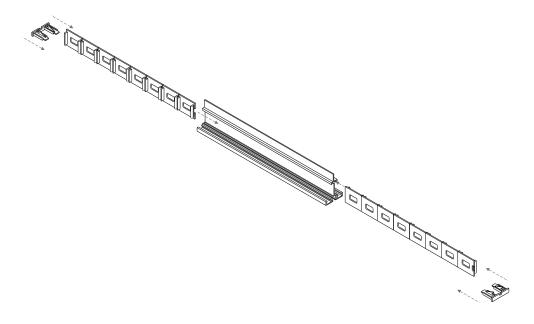
2. Drill a 3mm hole close to the edge of the Suspended Edge Strip Extrusion (same on both Sides of the Suspended Sign) to hang the sign from.
