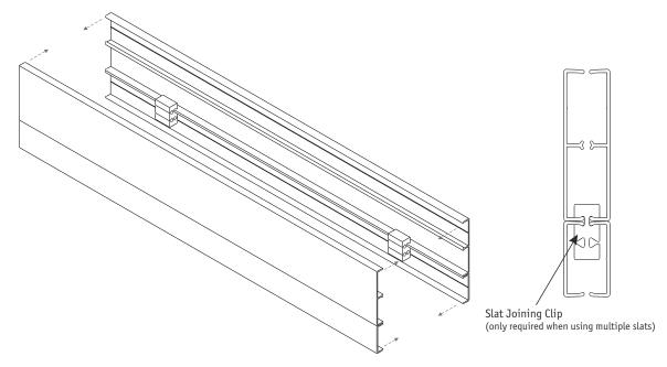
2. Push the Projecting Slat End Caps into the ends of the K'nect slat Extrusions (this may require some force). Leave one of the caps sitting out by 1.5mm for next step.
