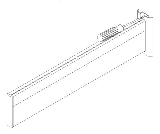
6. Slide the Projecting Base End Caps on the top and bottom of the Base Extrusion.
