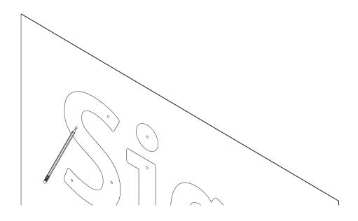
2. Now screw the female section of the Plastic Locators to the wall in the position of the hole marks.
