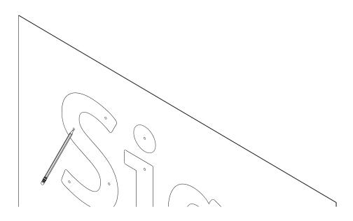
2. Now screw the female section of the nickel connector to the wall in the position of the hole marks making sure not to over tighten as the locator will be required to spin.
