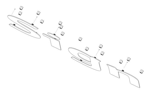
4. Turn the female section of the locator, which will tighten onto the male section on the letter. ( A Spanner may be required )
