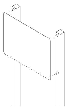
4. Screw the Front Section of the Stand off Connector through the holes to secure the panel into place.
