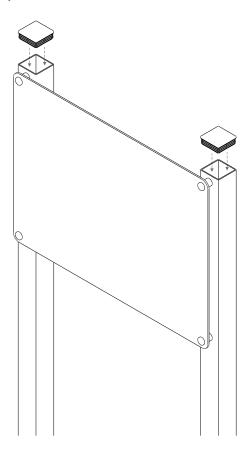
6. Now you can mount your signage into the ground. (No Steel baseplates required on square posts). The Corniche Post mounted sign is best mounted complete to make sure the post are in the correct position for the Locators. (Please see website for further instructions)
