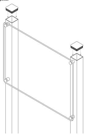
6. Now you can mount your signage into the ground. (No Steel baseplates required on square posts). The Corniche Post mounted sign is best mounted complete to make sure the post are in the correct position for the Locators. (Please see website for further instructions)
