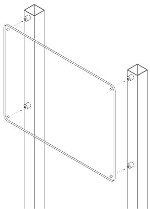
4. Screw the Front Section of the Stand off Connector through the holes to secure the acrylic panel into place.
