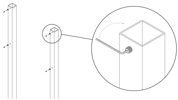
2. Screw the Middle Section of the Stand off Connector to the Back section by hand.
