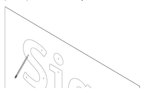
2. Now screw the female section of the Plastic Locators to the wall in the position of the hole marks.
