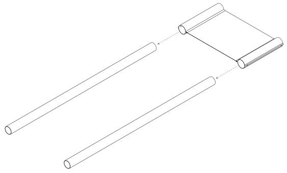
2. Place the Grub Screw into the As760 Extrusion and tighten them to the post.
