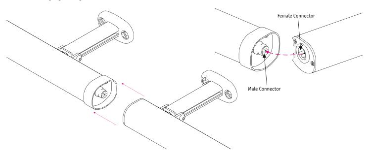
4. Tighten the Grub Screws in the Slider Bracket to clamp the Troughlights into place.
