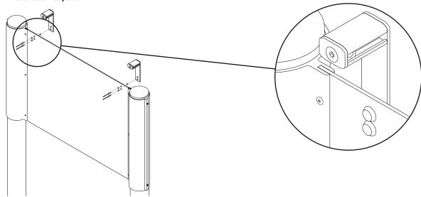
2. Slot the sliders (mounted on the troughlight) over the plate bracket arms and bolt into place using the M6 Bolts
