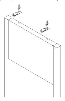
2. Slot the sliders (mounted on the troughlight) over the tray bracket arms and bolt into place using the M6 Bolts
