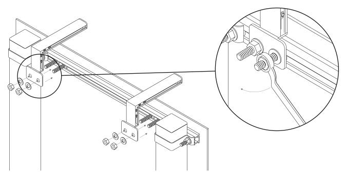
2. Slot the sliders (mounted on the troughlight) over the Channel bracket arms and bolt into place using the and external tooth washers / M6 Bolts
