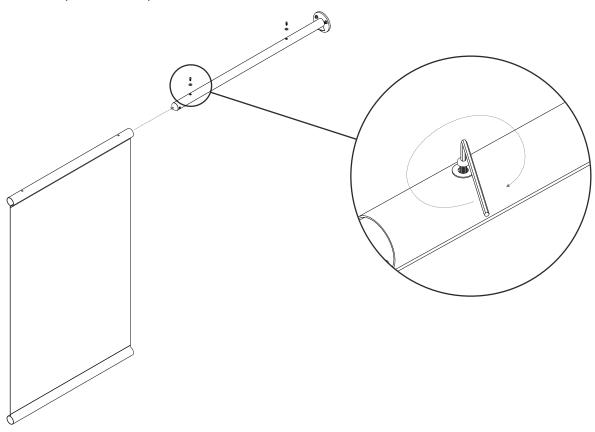
4. Slide the Middle Post (No Baseplate) into the bottom slot of the banner and stop it from sliding out using the M6 Eyebolts.
