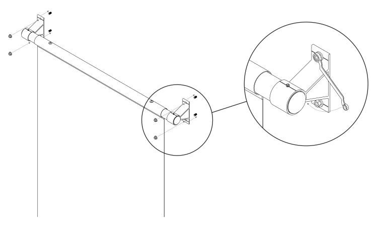
4. Slide the Middle Post (No Baseplate) into the bottom slot of the banner and stop it from sliding out using the M6 Eyebolts.
