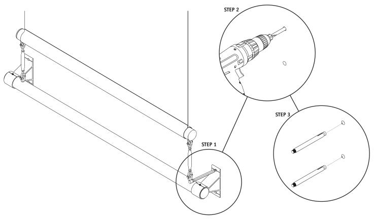
8. Slot the Bannerfast 180 Bottom Post and Brackets onto the sleeve anchors and tighten into place. Then adjust the rigging screws to create tension on the banner
