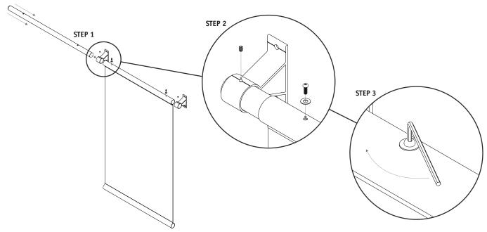
2. Mark the position of the Top post and bracket (Step 1), drill the holes for the Anchor Bolts (Step 2) Then place the Sleeve anchors into the holes (Step 3)
