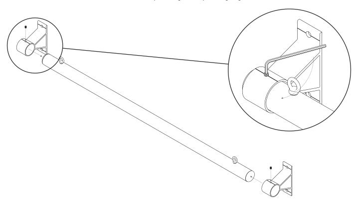
6. Connect the Bottom post to the middle post using the rigging screws (leaving the tension on the rigging screws loose).
